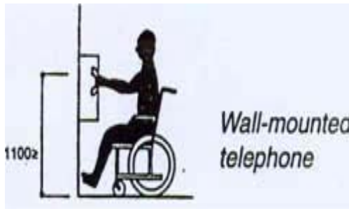
Fig-3. Telephone Stand & Wall Mounted Telephone
