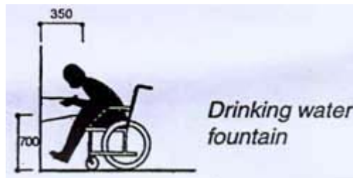
Fig-2. Drinking Water Fountain
